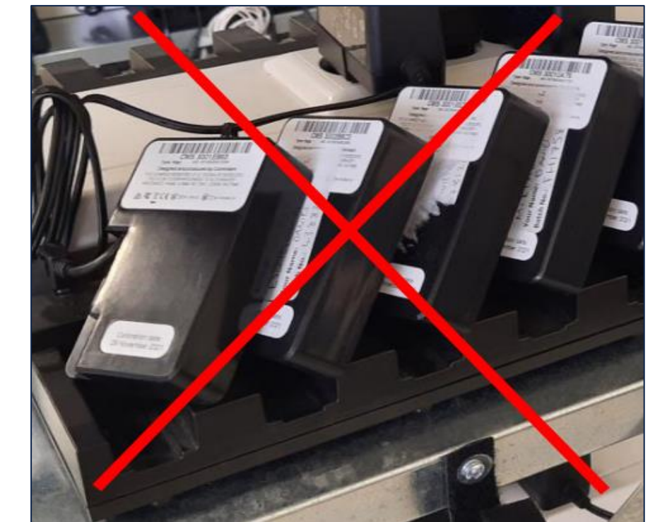
Loggers standing incorrectly in a charging station.
